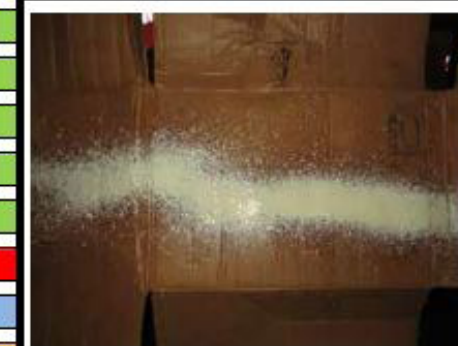
LUBRICANT SPRAY APPLICATION PATTERN
